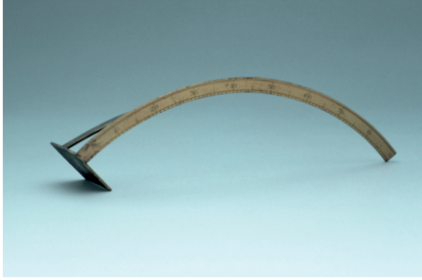
Figure 9: A Quadrant Scale, c. AD 1700.
